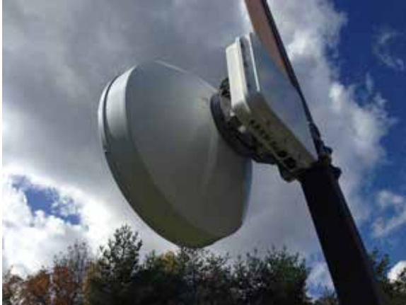
With high capacity and high speeds, wireless data communication links can leap across chasms in space to connect line-of-sight buildings at distances of several kilometers using highly directional, pencil-thin beams that prevent interference and strengthen security.
