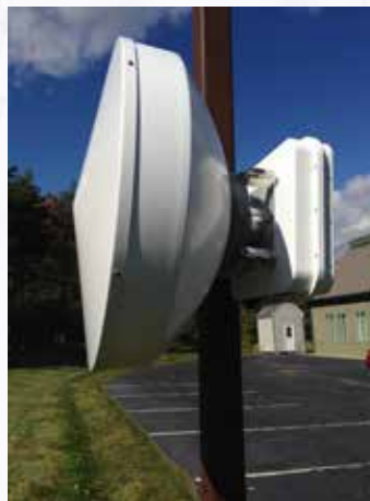
Expanding upon the improved functionality of wireless is the recent development of dual-capacity MMW wireless in a single polarization that only requires one antenna.
