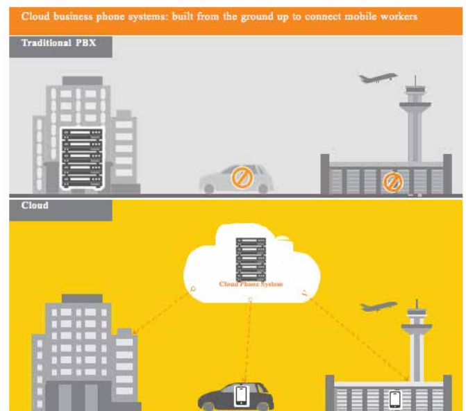
Figure 1: Moving up: With full-featured PBC functionality hosted in the cloud, workers on the go enjoy the same business desk phone features – such as extension dialing and direct voicemail access – as office staff.
